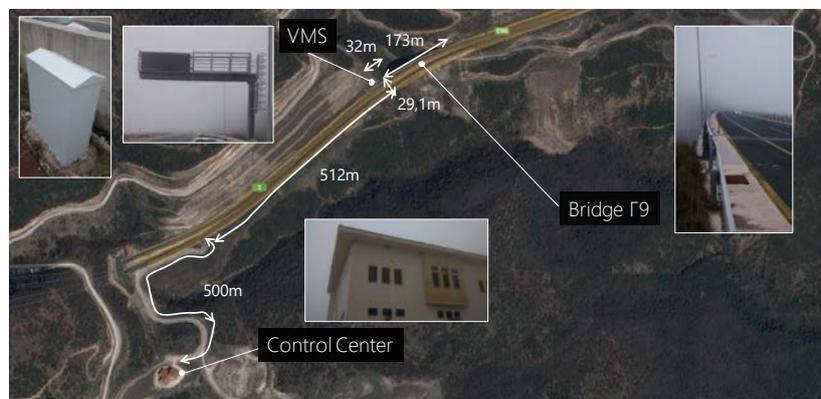
Figure 8: Layout of the monitoring scheme installed to G9 Egnaria Motorway bridge
