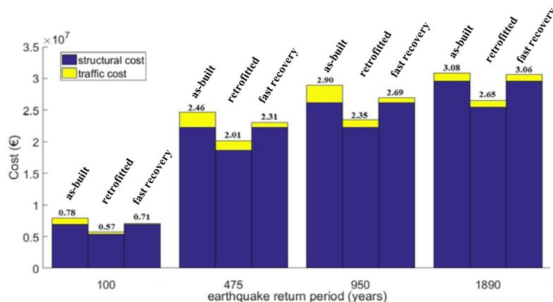
Figure 7: Expected costs for the four seismic scenarios for the case of the “as-built” network and the two risk mitigation strategies
